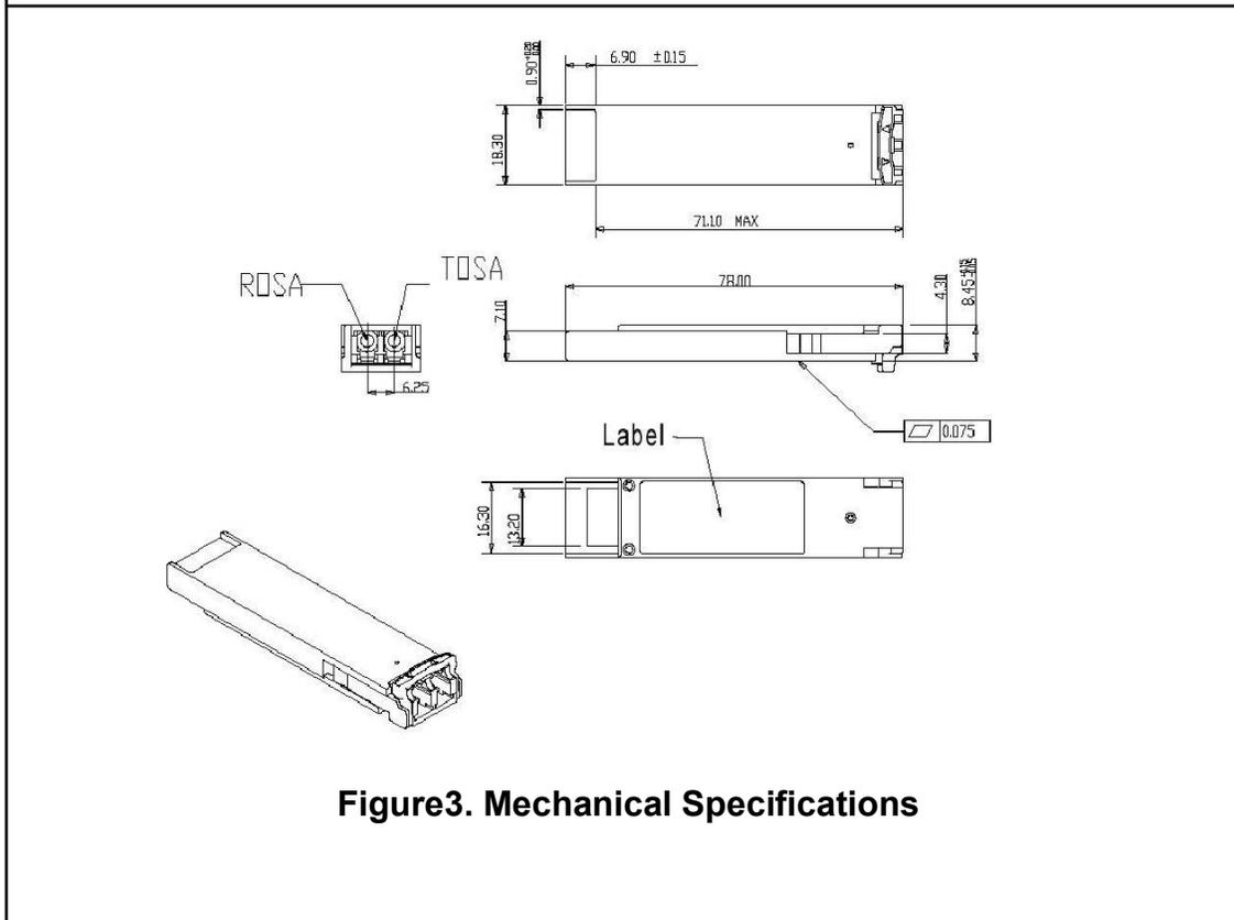
**Figure3. Mechanical Specifications**
